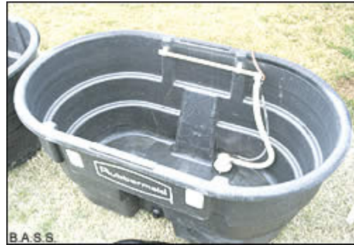
A bilge pump, hose and spray bar provide water circulation and aeration. A more efficient system uses a larger pump and several spray nozzles around the tank that both aerate the water and provide locations for contestants to refill their weigh-in bags.
